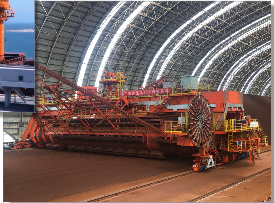
MCR on drum reclaimer for Caofeidian iron ore storage ThyssenKrupp, China
