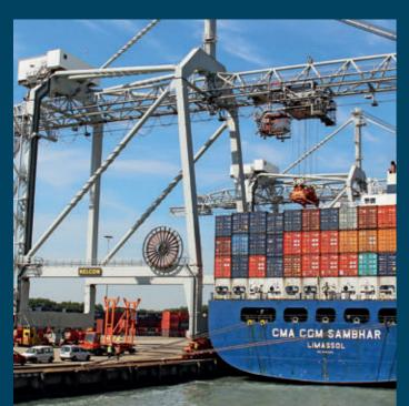
A wide range of rail mounted loading and unloading machines of each size installed at berths enable efficient handling of bulk goods. Motorized cable reels by Hartmann & König are designed to accomplish numerous tasks that include horizontal movements, distances up to 60 m, acceleration of  $0.2 \, \text{m/s}^2$  and slip ring bodies of up to 1000 A.
